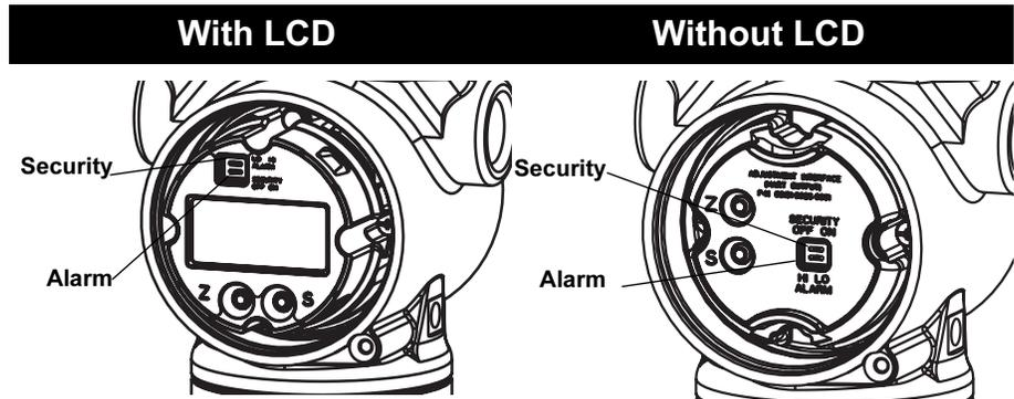
Slide the security and alarm switches into the preferred position by using a small screwdriver.
