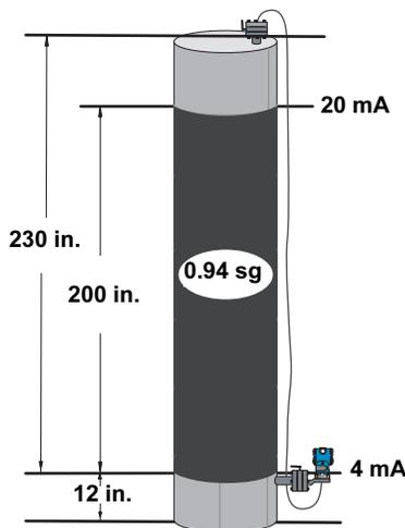
A differential transmitter is used in a level application where the span is 188 inH<sub>2</sub>O (200 in. \* 0.94 sg). Once installed on an empty tank and taps vented, the process variable reading is -209.43 inH<sub>2</sub>O. The process variable reading is the head pressure created by fill fluid in the capillary. Based on Figure 3-3, the Scaled Variable configuration would be as follows:
