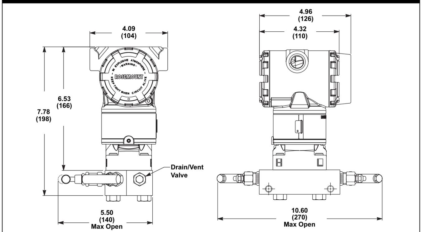
**Coplanar Flange Mounting Configurations with
