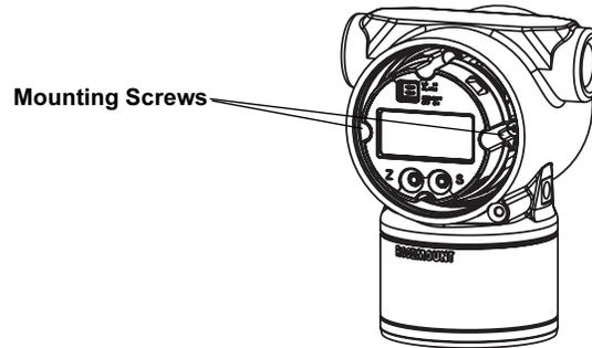
3. Rotate the LCD counterclockwise slightly to disengage snap fit.
