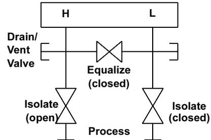
Next, open the center (equalize) valve(s) to equalize the pressure on both sides of the transmitter.
