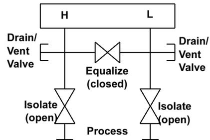
To zero the 3051, close the isolate valve to the low pressure (downstream side) of the transmitter first.
