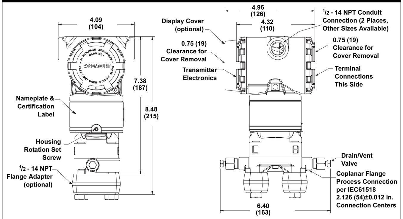
**3051C Coplanar with Rosemount 305 Coplanar Integral Manifold**
