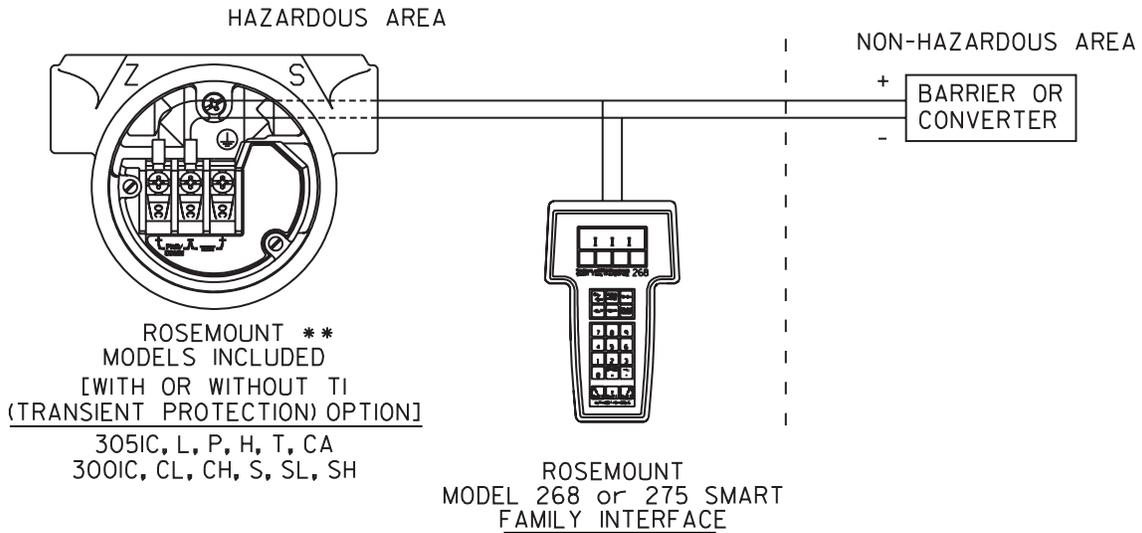
\*\* FOR THE LOW POWER OPTION, SEE PAGE 4 FOR THE CIRCUIT CONNECTION WITH BARRIER OR CONVERTER. FOR FIELDBUS OPTIONS("F" or "W" OUTPUT CODE), SEE PAGE 5 FOR PARAMETERS AND CIRCUIT CONNECTION TO BARRIER.
