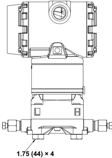
**TRANSMITTER WITH FLANGE ADAPTERS AND FLANGE/ADAPTER BOLTS**
