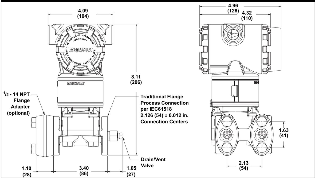
**3051C Coplanar with Rosemount 305 Traditional Integral Manifold**
