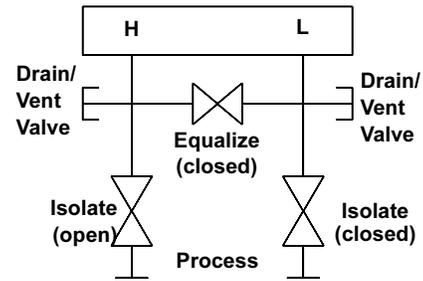
Next, open the isolate valve on the low pressure side of the transmitter.
