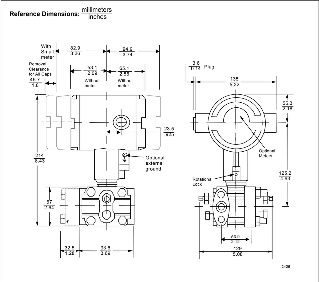
**Figure 5**—Typical mounting dimensions for dual-head models STG944 and STG974 for reference
