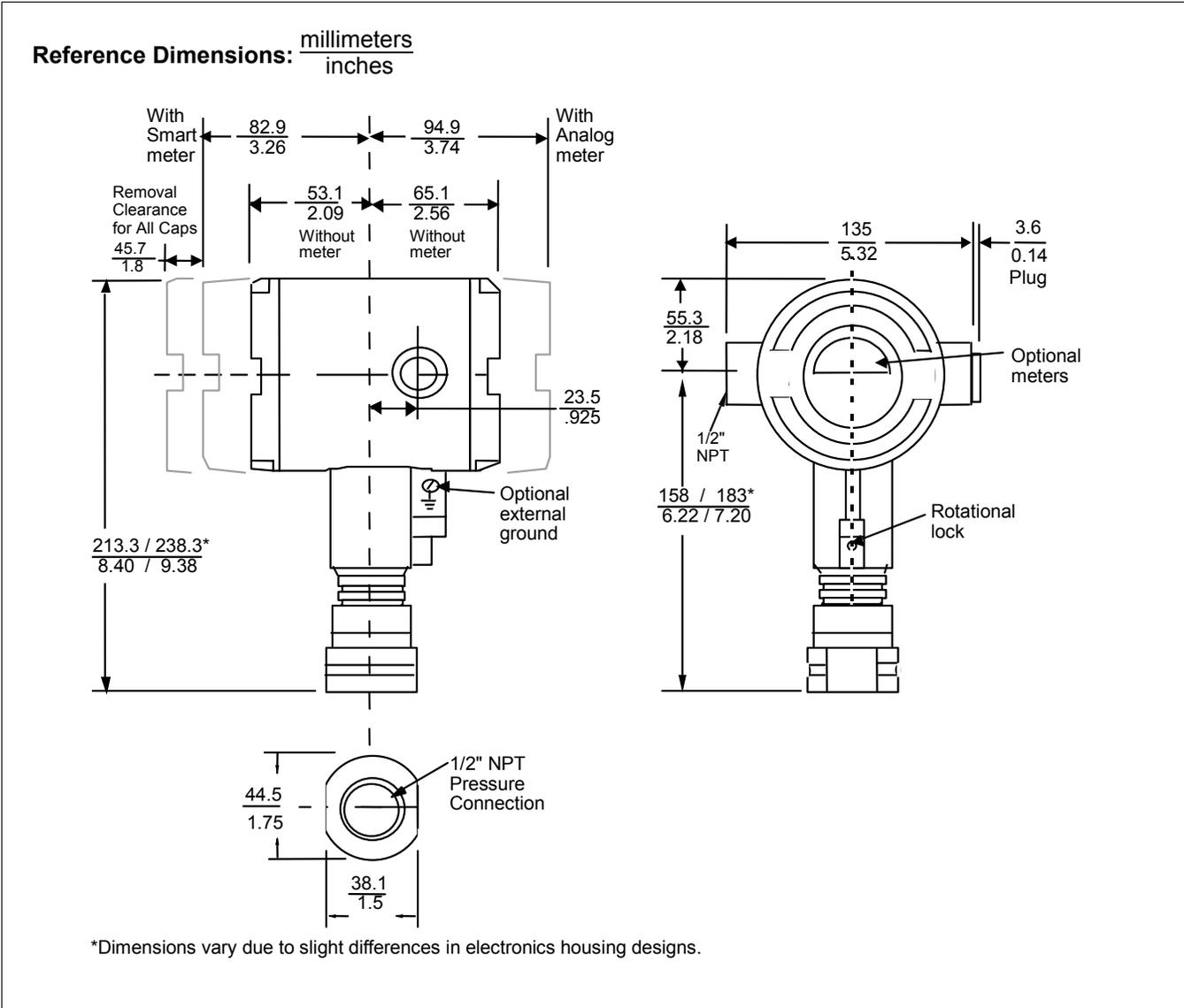
**Figure 6**—Typical mounting dimensions for in-line models STG94L, STG97L, STG98L, and STG99L for reference
