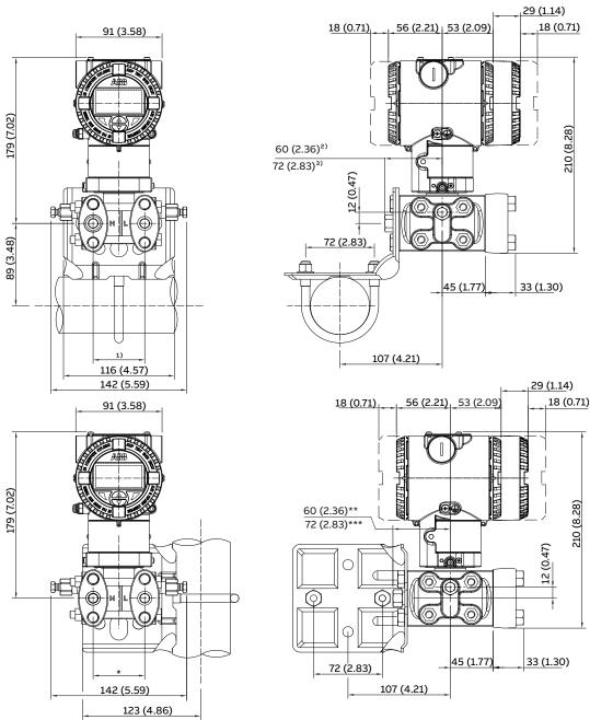
Transmitter with mounting bracket, for vertical or horizontal mounting on 60 mm (2 in) pipe pipe
