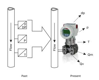
Figure 1: Flow measurement - past and present
