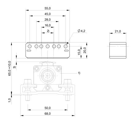
1) not included in scope of delivery, 2) Lateral offset, 3) Distance to BTL
