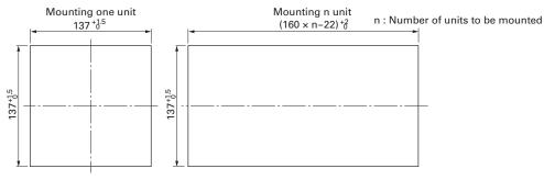
Do not use the water proof packing in case of mounting n unit
