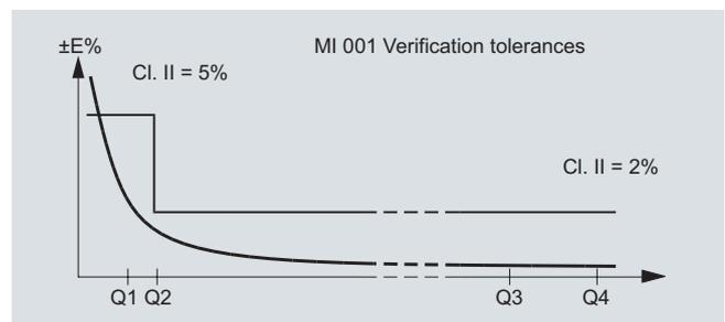
MAG 5100 W MI-001 verified and labeled products at a given Q3 and Q3/Q4 = 1.25 and Q2/Q1 = 1.6 measuring ranges see table below:
