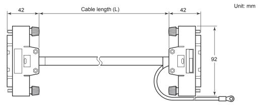
AKB331: L = 1 m, 2 m, 3 m, 5 m, 7 m or 10 m, up to 50 m in 5 m increments
