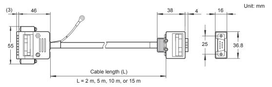
Note: An FG connection wire is attached to the other side connector of the AKB131 and AKB132 cables.
