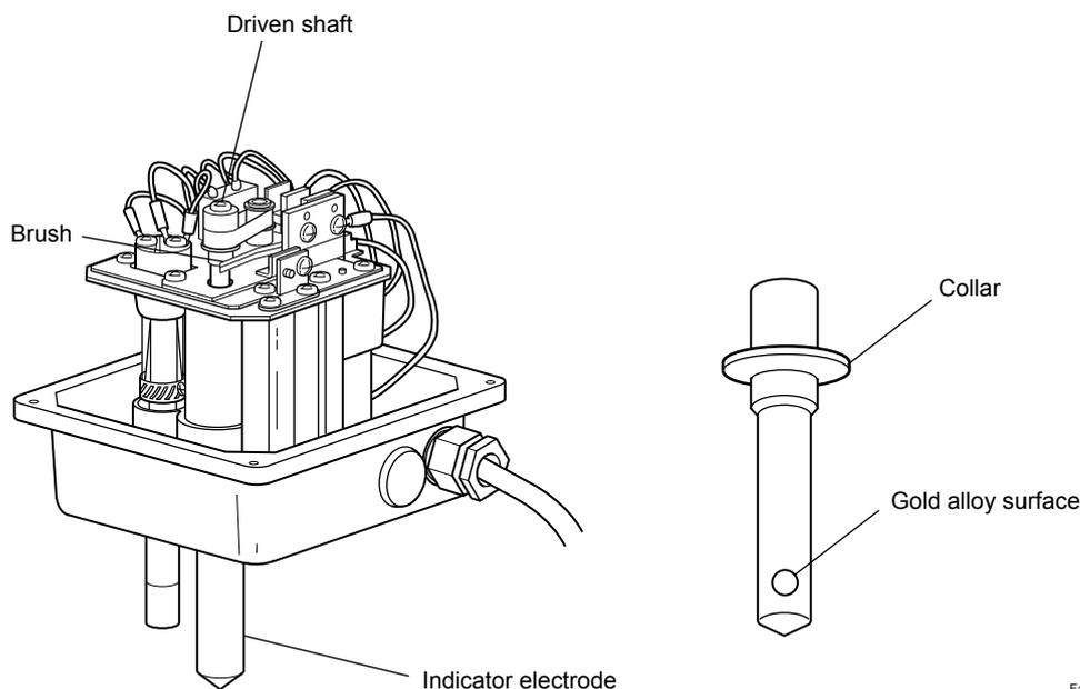
**Figure 4.8 Appearance of electrode mechanism block and Indicator electrode**
