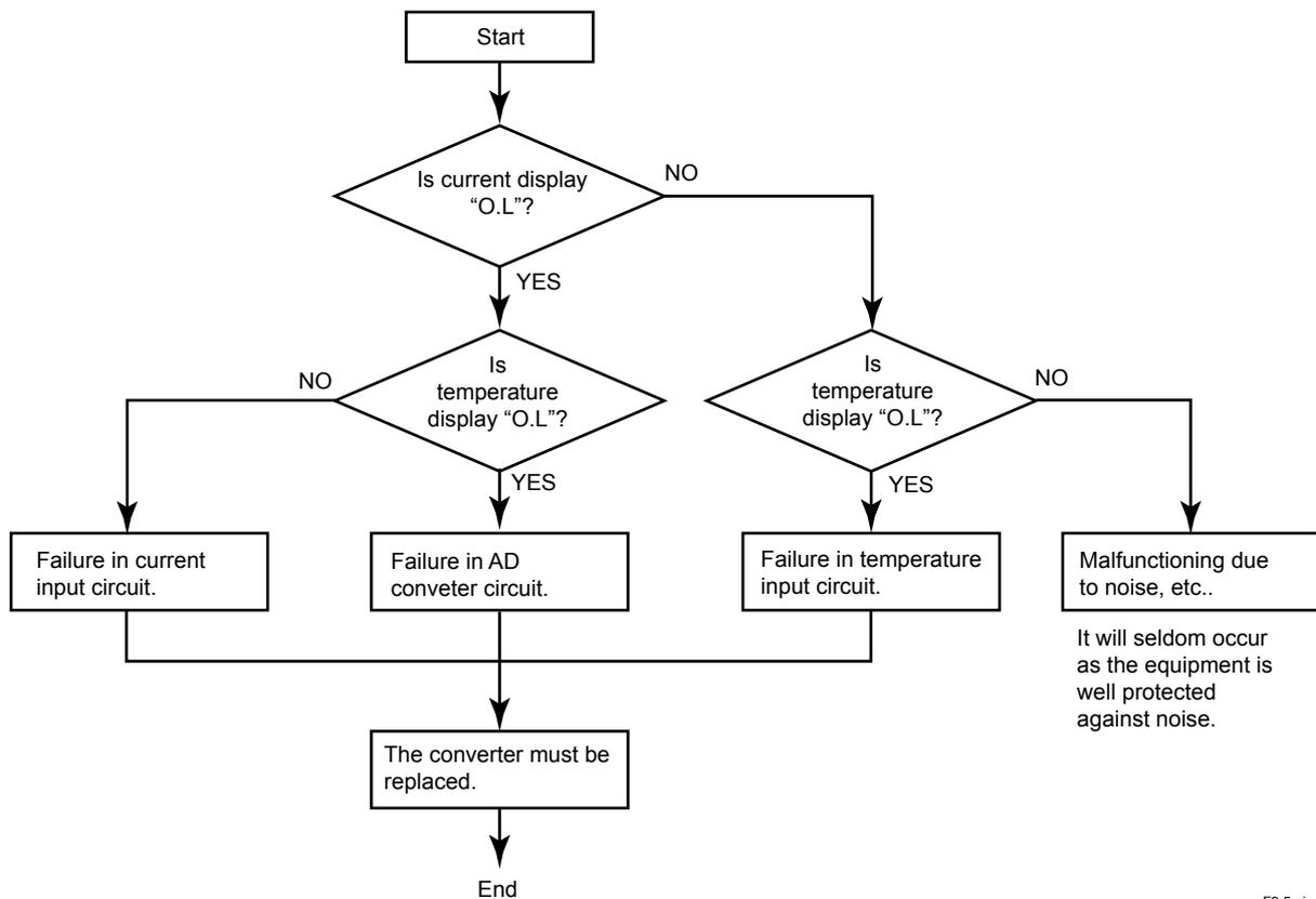
Figure 9.5 Converter Failure Inspection Flow Chart
