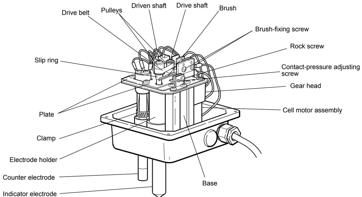
Figure 8.7 Electrode Mechanism Block
