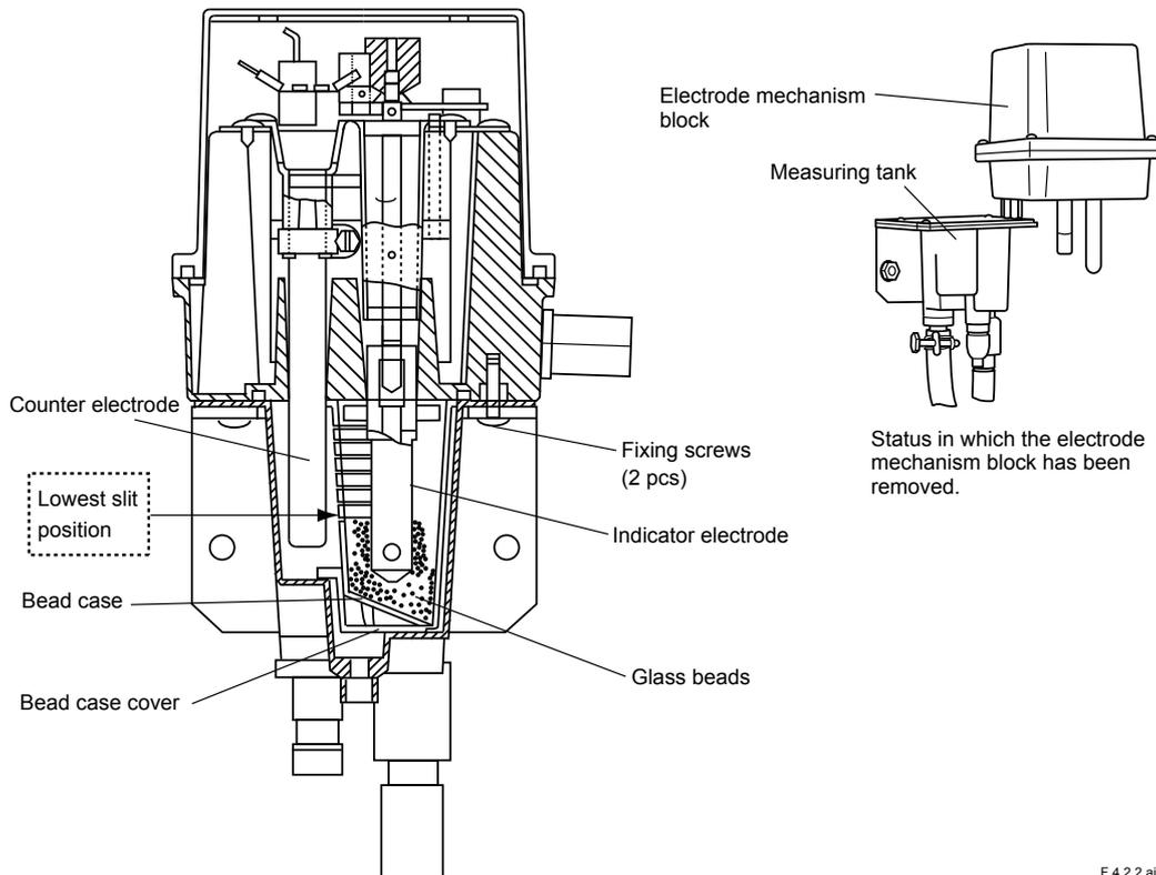
Figure 4.4 Detector Construction
