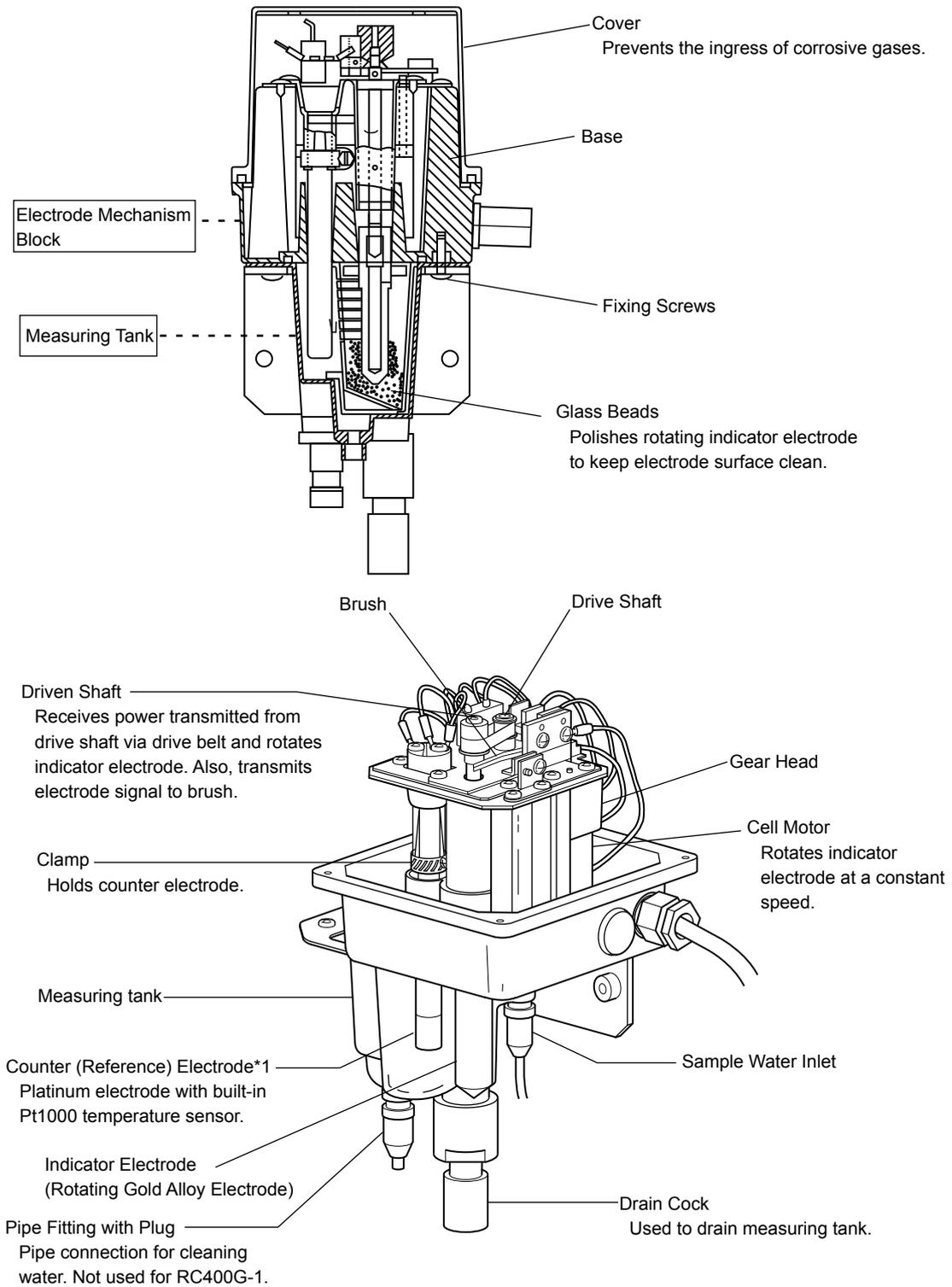
\*1 In the case of combined chlorine insensitive version, silver chloride electrode with built-in Pt1000 temperature sensor is used.
