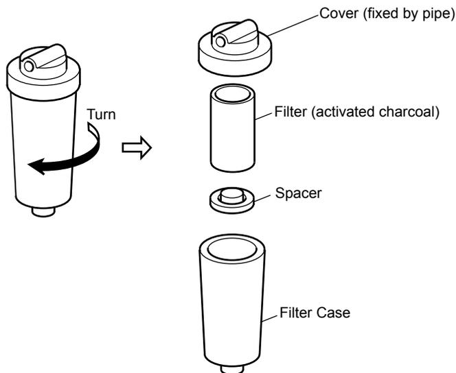
Figure 8.8 Replacing Activated Charcoal Filter
