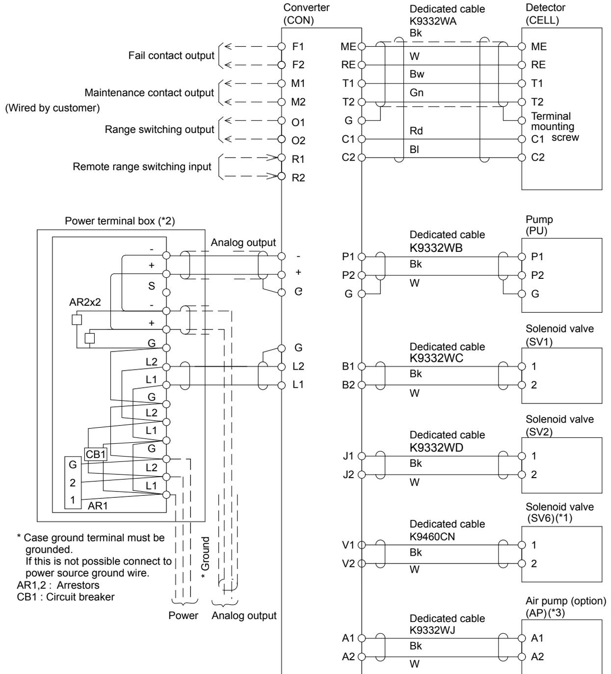
\* Case ground terminal must be grounded.
