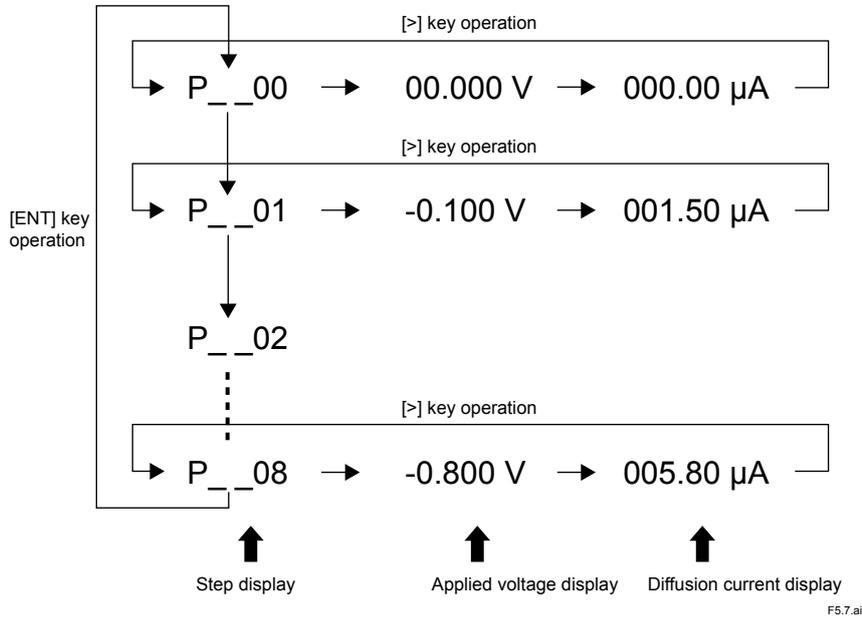
Figure 5.7 Key Operations for Displaying Plateau Characteristics
