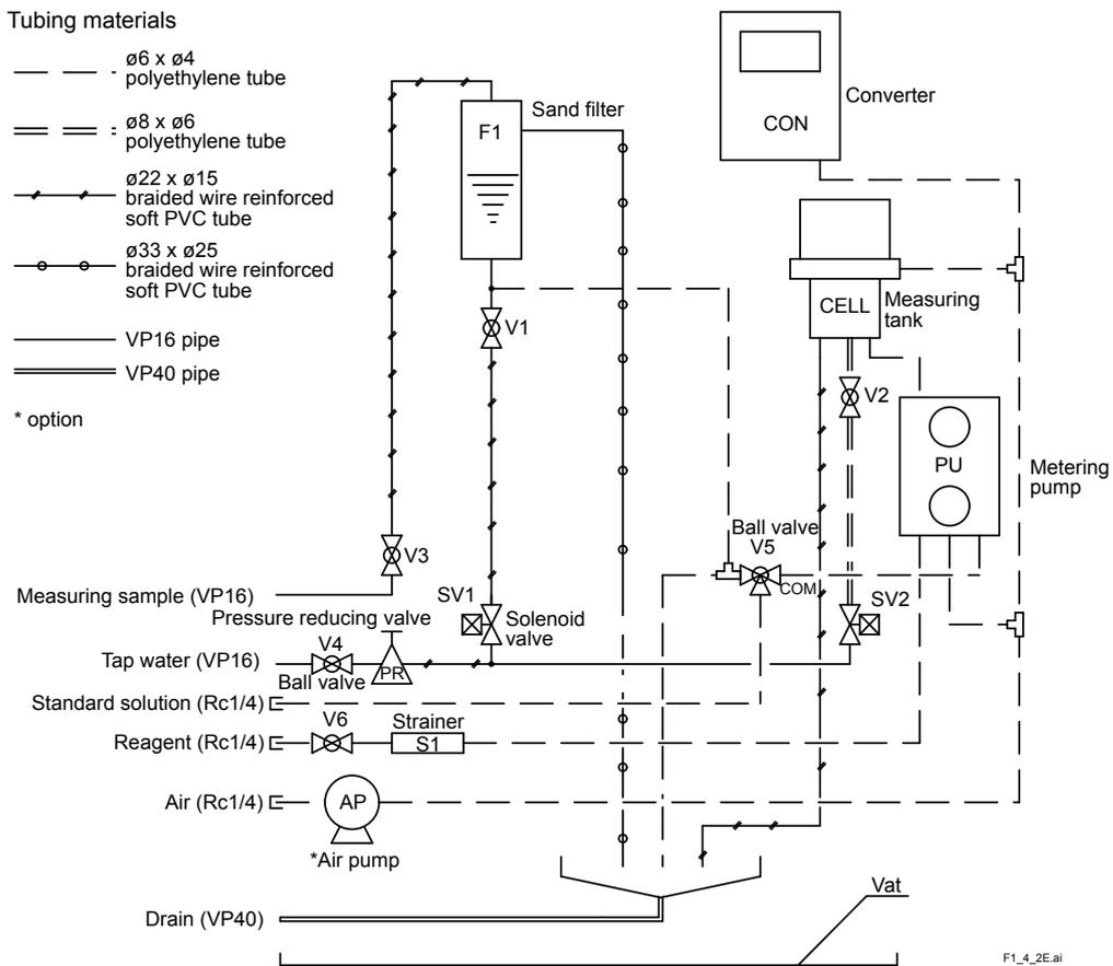
**Figure 3.2.2** Tubing Diagram of RC400G-2
