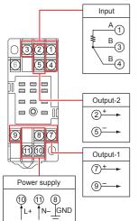
The wiring resistance of input terminals 1 and 3 should be the same.
