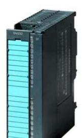
SIPLUS S7-300 SM 332 4AO U/I -25...+70°C with conformal coating based on 6ES7332-5HD01-0AB0 . Analog "output SM 332, isolated, ""4 AO," "U/I; diagnostics;"" resolution" 11/12 bits, 20-pole, removing and inserting possible with active backplane bus
