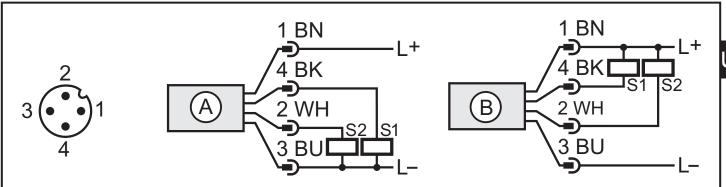
A: SI5002; SI0521 (positive switching); B: SI5003 (negative switching)
